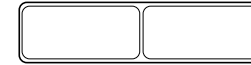
65 x 16 x 1.4mm SLAT with Centre Support Gusset (Lengths: 1800mm; 2400mm; 3600mm)
