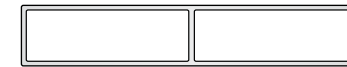
90 x 16 x 1.4mm SLAT with Centre Support Gusset (Lengths: 1800mm; 2400mm; 3600mm)
